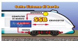
The train speed control systems (TSCS) is a safety system that helps the driver and provides the control of the maximum speed permitted instant by instant, in relation to constraints put in place by signalling, the infrastructure's characteristics and the train's performance both in normal and deteriorated conditions. The system can be used on electrified lines on main, complementary and hub networks and on single or double tracks. It is certified for up to maximum speeds of 250 km/h.
